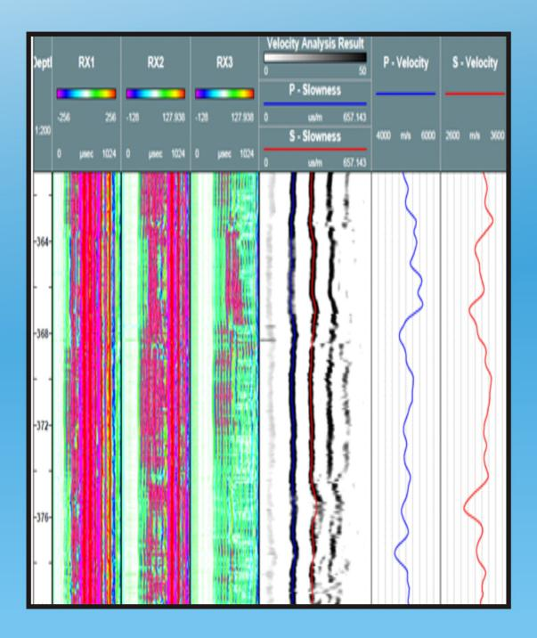
Because the total transit time from the transmitter to the receiver includes the path through the borehole fluid + formation + borehole fluid, borehole compensated (two or four receiver) logging tools are used. Borehole compensation is accomplished mathematically by subtracting the borehole transit time. It gives information resulting young's modulus, bulk modulus, shear modulus, Poisson ratio, and Porosity.
