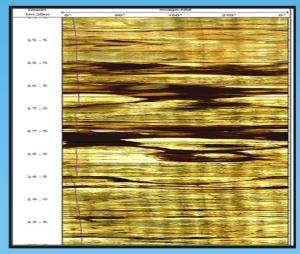
Similar to the acoustic televiewer but using visible light optics, the **OPTV** probe provides a continuous detailed and orientated 360° true color image of the borehole walls using a unique optical imaging system. This can be rapidly interpreted, using data from the internal orientation module, to obtain a complete feature analysis that includes dip, strike, and frequency and fracture aperture.
