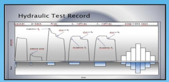
The hydraulic stress tests were conducted in close agreement with the ISRM - standard. The in- situ stress field components have been widely recognized as basic parameters in the engineering design of underground constructions. The most common method of measuring in-situ stresses is hydraulic fracturing.
