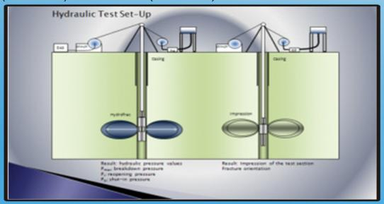
The shut-in pressure equals the rock stress, at which the hydro fracture closes completely under the action of the stress acting normal to the hydro fracture plane. In a vertical test hole the new induced hydro fracture is expected to be vertical and perpendicular to the minimum horizontal stress.
