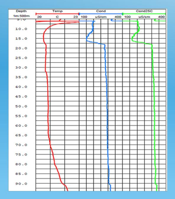
The borehole fluid conductivity is measured using a seven electrode mirrored wenner array for measuring borehole fluid conductivity. The conductivity array is an internal cylindrical array open at the bottom of the probe. Borehole fluid passes by the array as probe is lowered in the hole. The array is completely shielded from the outside borehole, so that only fluid conductivity is measured.
